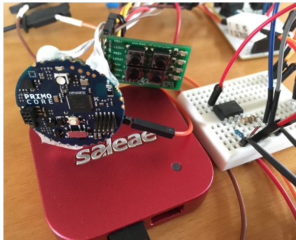
Figure 8: Experimental setup: Primo Core with keypad, amplifying circuit and logic analyzer
